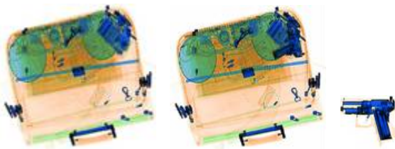
Figure 1: Example of an x-ray image of a passenger bag. The image on the right contains the prohibited item depicted separately on the bottom right.
